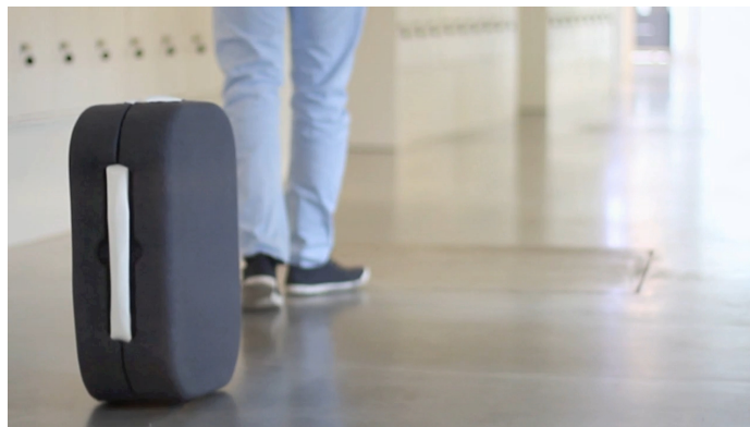
Figure 1.2: Hop! following suitcase ( García , 2012). The suitcase utilizes bluetooth receivers to track a Bluetooth beacon from the leader's phone.
