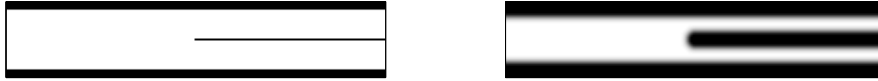
Figure 5.2: Example of human presence probability map. (Left) Occupancy map from a simulated corridor with a divider in the middle (white – free space, black – obstacles). (Right) human presence probability map (white – high probability, black – low probability)
