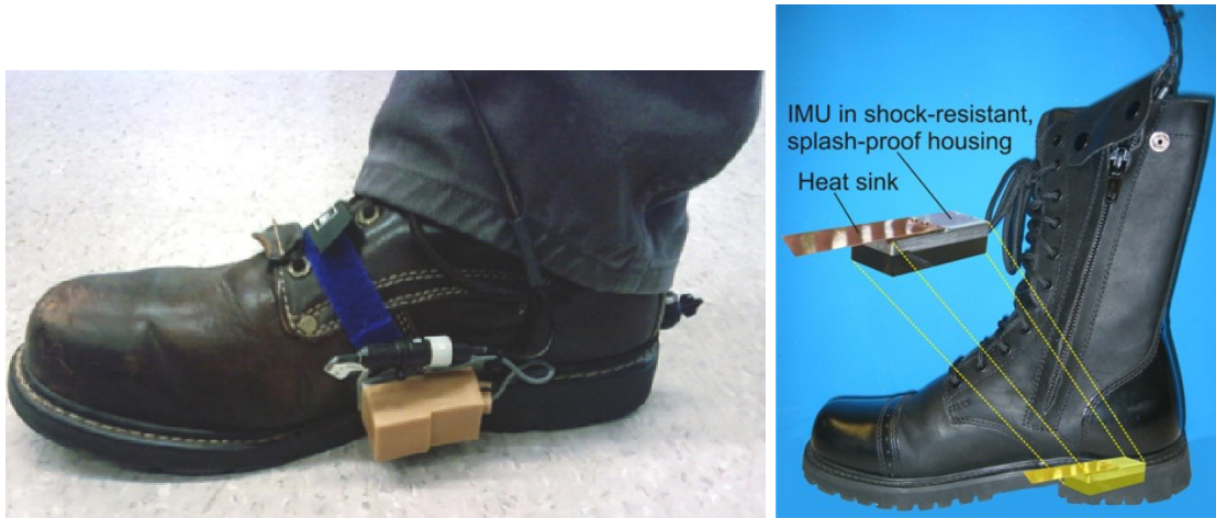
Figure 2.1: The foot-mounted IMU of the PDR system has two mounting options. (a) Side-mounted IMU (the IMU itself is covered by the beige-colored thermal insulation). (b) In-heel IMU with temperature controlled, shock resistant housing
