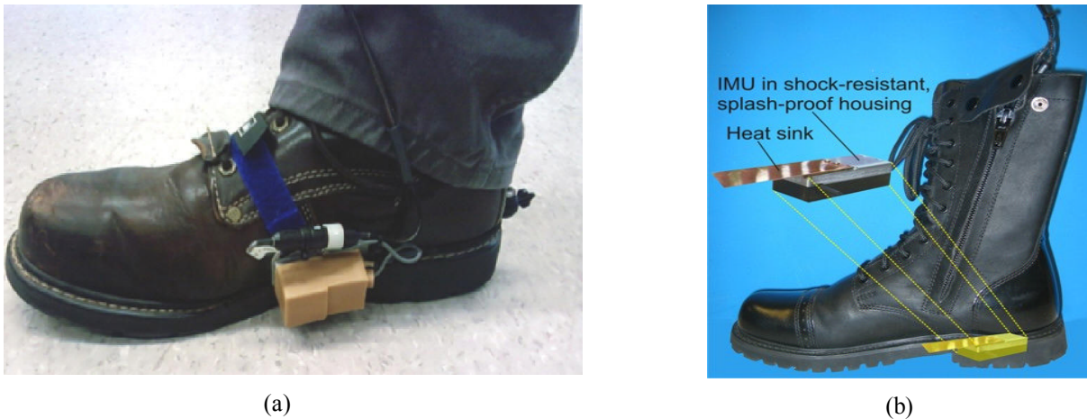
Figure 1. The foot-mounted IMU of the PDR system has two mounting options. (a) Side-mounted IMU (the IMU itself is covered by the beige-colored thermal insulation). (b) In-heel IMU with temperature controlled, shock resistant housing
